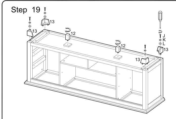
Attach legs (13) to bottom panels (3,4) using bolts (J), spring washers (K) and washers (L) as guides. Screw support legs (12) into bottom panel (11).
